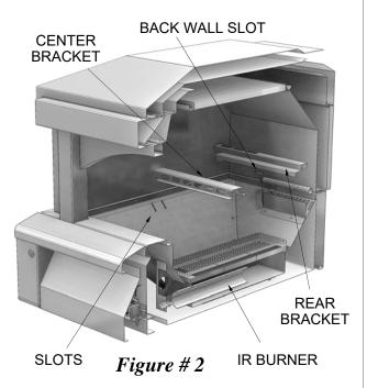
Once the Hearth Stones are installed inside the oven, the Log Support Tray can be inserted into the slots that can be found at the bottom of the oven cavity back wall. (**See figure # 2**).
