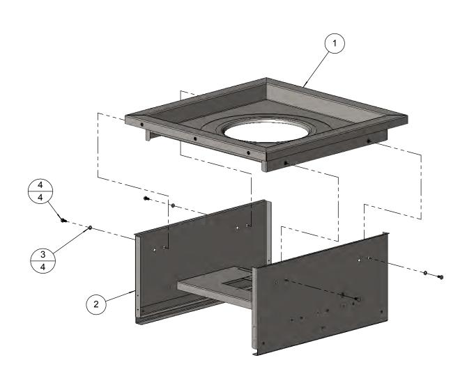
**NOTE:** AGVPC UNITS BUILT AFTER 07/2009 HAVE BODIES BUILT WITH TWO ASSEMBLIES, TOP (510-0448), ITEM 1 AND BOTTOM (510-0449), ITEM 2, MAKING THE TOP OR BOTTOM ASSEMBLIES REPLACEABLE BY THEMSELVES.
