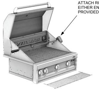
ATTACH ROTISSERIE MOTOR TO EITHER END USING THE HARDWARE PROVIDED
