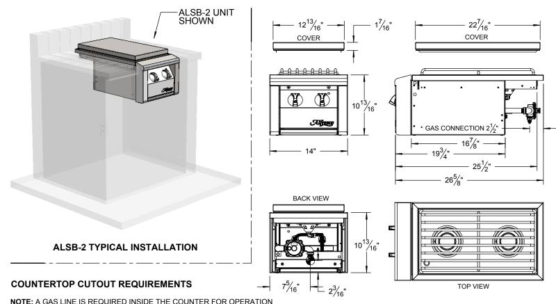
**NOTE:** A GAS LINE IS REQUIRED INSIDE THE COUNTER FOR OPERATION FOR LP-GAS SETUP SEE NOTE AT RIGHT. IT IS RECOMMENDED THAT A FLEXIBLE HOSE IS USED FOR NG-GAS SETUPS TO EASE INSTALLATIONS.
