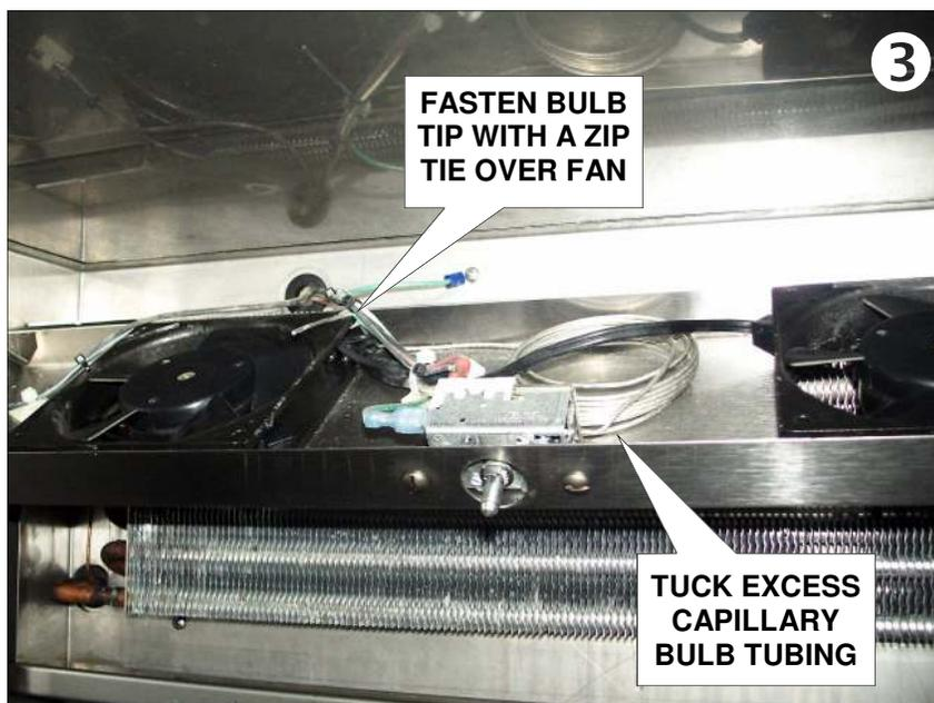
Place the BULB TIP over the left evaporator fan (approx. 1" exposed over fan blades) and fasten to the fan corner mounting hole with a zip-tie.
