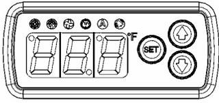
The Renau™ control used by *Alfresco™ Refrigerators* has been custom programmed for our units. The controller needs to be commissioned upon installation in order to operate correctly and control temperature.
