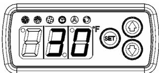
Once the SET key is pressed, the display will show the number 30. That is the current SETPOINT temperature.
