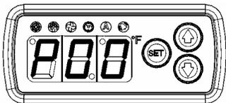
After 10 seconds, the letters P and numbers 00 will appear flashing. This indicates the unit is set for PROGRAM # 00
