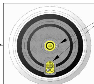
(2) Orifices are Located inside burner body. (2002 or older models only)
