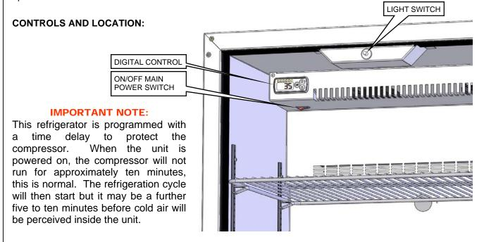
Switch the unit ON using the main ON/OFF power switch. Immediately after the unit is switched on the cabinet light and inside evaporator fans will start operating. Check the temperature setting which has been set at the factory to 35°F.
