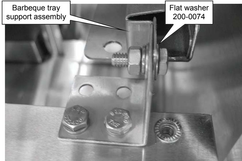
Note: The above two views show the rear left side of the barbecue being secured to the cart. To secure the rear right of the barbecue to the cart, the second mounting bracket (130-1631) must be attached in the same manner but with the bracket rotated 180°, thereby using the three holes not used when securing the rear left.
