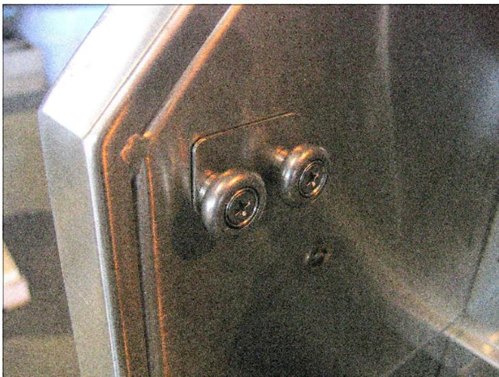
**SPIT ROD SPACER LOCATED PROPERLY IN THE REAR HOOD ASSEMBLY AFTER INSTALLATION**
